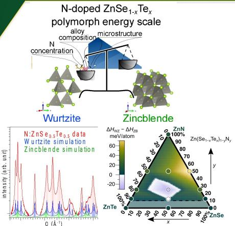
(left) Wide-angle synchrotron x-ray diffraction data of a phase pure wurtzite film. (right) Polymorph energy calculations indicate N-substituted ZnSe<sub>0.5</sub>Te<sub>0.5</sub> compositions favor wurtzite.
